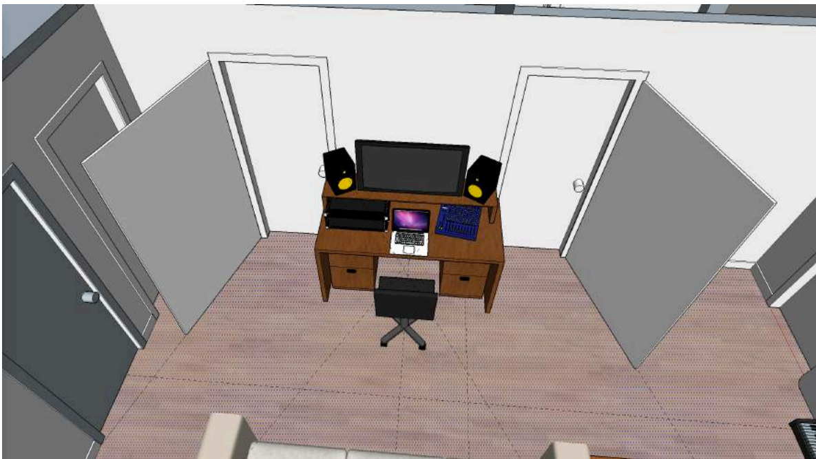
The beginning of my modular reflection-free zone plan, built around simple panels angled on each side of the listening position.
