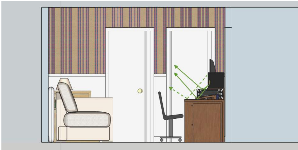
Side view, ray trace with speakers inverted (solid lines), note improvement vs upright (dashed).
